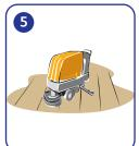
Remove slurry with wet pick up machine or mop.
