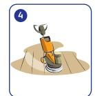
Using rotary machine, scrub using a stripping grade pad.
