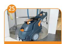
Store the machine after working and leave the covers open to allow air to circulate.
