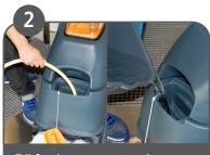
Fill fresh water into solution tank with a coupling hose or by using a bucket.
