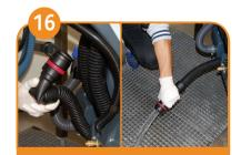
Empty the waste water tank by using the hose with the red mark
