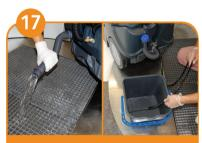
Empty fresh water into a sink through the blue marked draining hose or into a bucket by using the additional draining hose.
