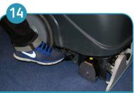
Lift-up the brush and suction unit by pressing the foot pedal.
