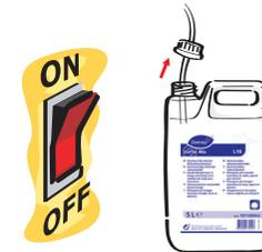
Switch off machine and wearing gloves and goggles remove feeder tube from empty container.
