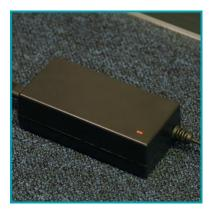
The charger LED light will be red during charging and will turn green when the battery pack is fully charged.
