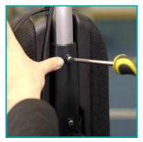
Place the handle bracket back into position and secure the two screws.
