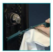
To install a new bag, slide the bottom of the green bag collar into the bag holder until it snaps into position. Push the top of the bag collar upward until the collar snaps into place on the vacuum.
