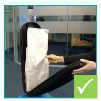
Unzip the bag compartment and check the vacuum bag is fitted.
