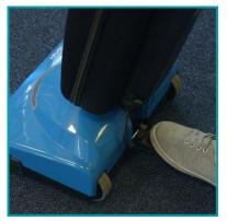
To recline the vacuum press the handle release pedal located on the back of the vacuum with your foot to recline the handle.
