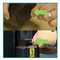
To charge the battery plug the AC cable into the charger and plug the DC cable into the charge point on the battery.
