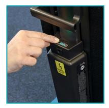
The battery life display is situated at the back of the machine. Press the button on the battery to illuminate the LED lights.
