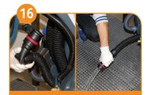
Empty the waste water tank by using the hose with the red
