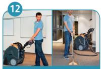
Clean the floor with the machine or by using a hand tool. The triggers on the handle will activate the brush and apply solution based on application mode. NOTE: The machine
