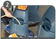
Fill fresh water into solution tank with a coupling hose or by using a bucket. Or fill using a dispensing system.
