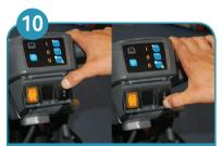
Choose the application mode you need. I. for encapsulation II for deep cleaning extraction NOTE: Vacuum will only turn on during II mode.
