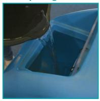
Fill the fresh water solution tank with mixed water and approved cleaning chemical according to the chemical manufacturer's instructions.
