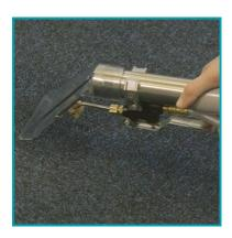
Operate the spray lever on the handle to dispense the cleaning solution whilst pulling the upholstery tool or wand backwards.
