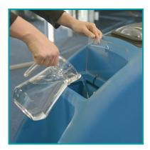
When solution spray ceases the solution tank is empty. Switch off the machine, empty the recovery tank and refill the solution tank.
