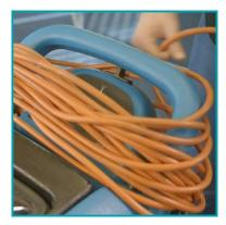
Wrap supply cord around handle ensuring that plug is not trailing on the floor.
