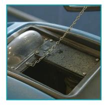
After a few passes, check the waste tank to see that no foam is present. Add extra defoamer if necessary.
