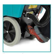
To lower the floating brush, press the foot pedal.
