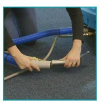
Attach the upholstery tool to both the vacuum and solution hose on the other end.
