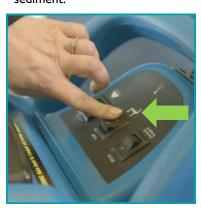
Turn on the PUMP switch. This will pump out any remaining solution.
