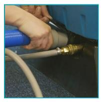
If using these accessories, connect the vacuum and solution hose to the front of the machine.
