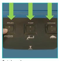
Switch on the vacuum motor, pump and brush switches.
