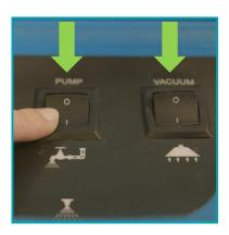
Switch on the vacuum motor and pump switch.
