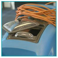
Store the machine with the recovery tank lid removed and store in a dry indoor area only.
