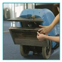
Check the vacuum and brush for debris. The brush should be raised for storage.
