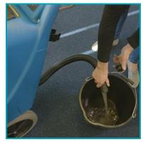
To drain the recovery tank, release the drain hose at the rear of the machine and empty into a bucket. Rinse out the tank with clean water to remove dirt and sediment.
