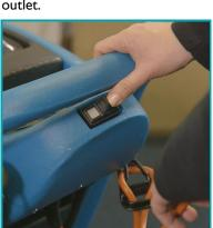
Press and hold the solution switch to apply the cleaning solution, whilst pulling the machine slowly backwards to clean the carpet.
