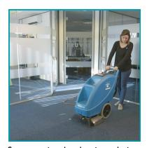
Stop spraying the cleaning solution about 30cm before the end of the cleaning pass to ensure all solution is vacuumed up.
