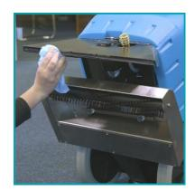
With both water tanks empty the machine may be tilted backwards to rest on the handle to facilitate cleaning. Wipe down the machine, including the underside of the machine.
