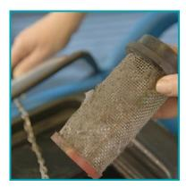
Regularly check the filter by removing and rinsing out any dirt or debris.
