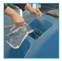
Add approx. ½ litre of clean water to solution tank to flush out the tank and pump. Once draining is finished, remove the drain hose.
