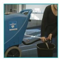
Make sure to empty the recovery tank when it is approximately  $\frac{3}{4}$  full. Do not refill the solution tank without emptying all the contents of the recovery tank first.
