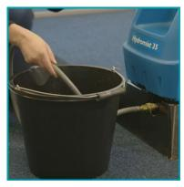
To drain the solution tank: connect the drain hose to the solution fitting at the front of the machine and direct the free end into a bucket.
