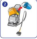
Pour solution into tank. Anti-foam is not required.
