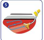
Extract the carpet using overlapping passes with the machine.
